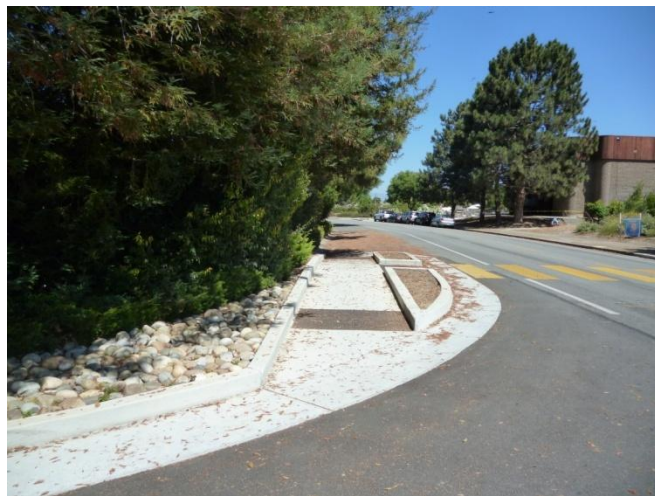
While crosswalks are best when they connect to a larger sidewalk network, sometimes a minimal treatment still works. Above, across from Blach Elementary, a bulbout provides visibility for crossing pedestrians.
