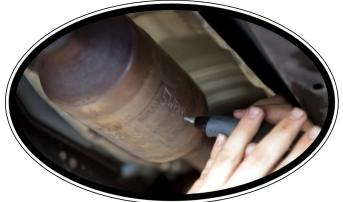
⇒ Etching a catalytic converter with your license plate or VIN number will assist police to help track the converter in the event it is stolen and recovered.
