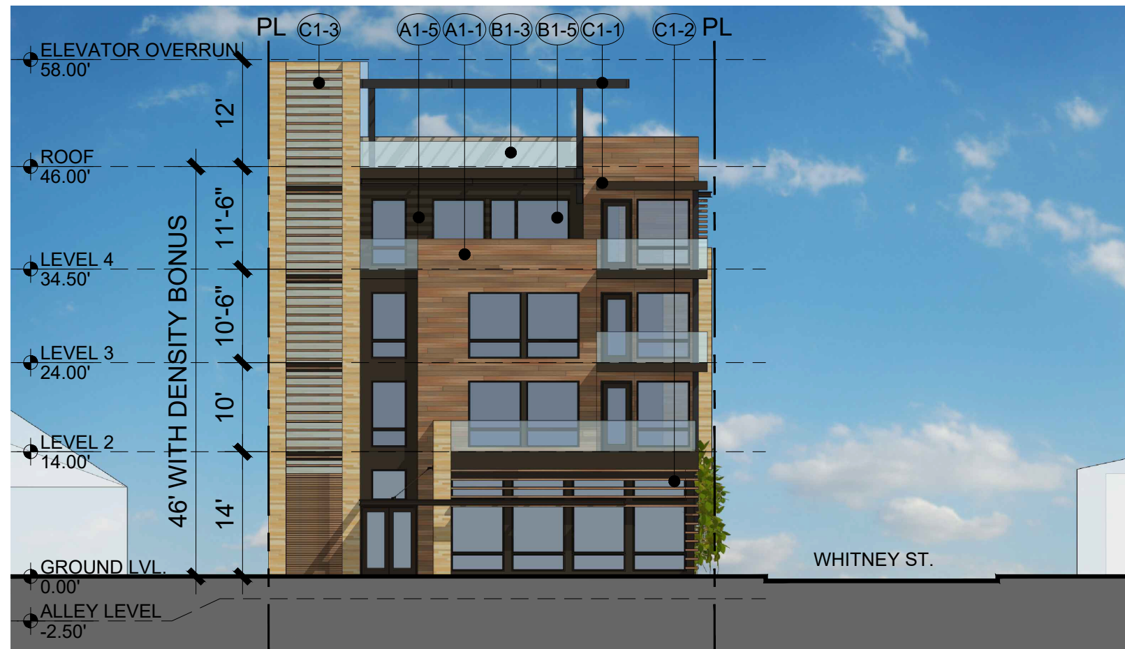
1ST ST. ELEVATION ② SCALE: 1/16" = 1' - 0" @ 11"x17"
