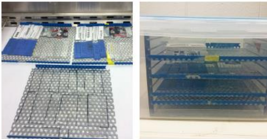
Figure 1. Inoculation of SARS-CoV-2 onto Test 3 materials (left). After inoculation, the extracted test coupons were placed inside the exposure chamber to control Temp and RH (right).
