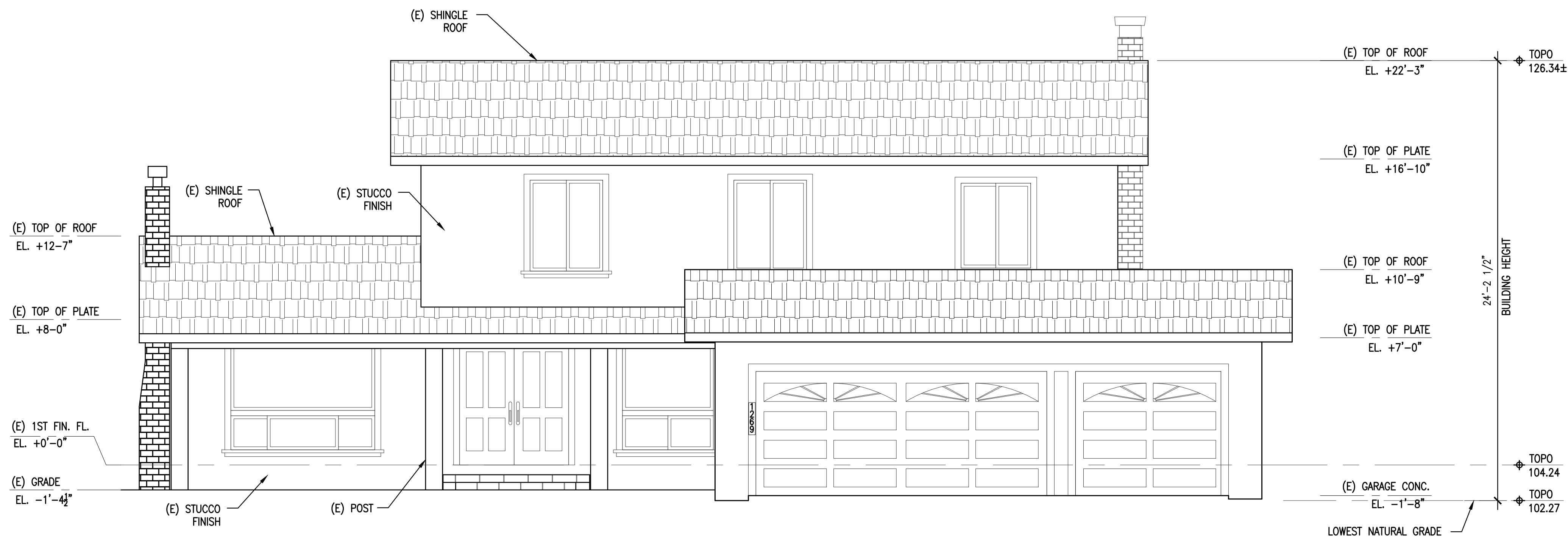
EXISTING FRONT EXTERIOR ELEVATION - SOUTH 1 1/4" = 1'-0"
