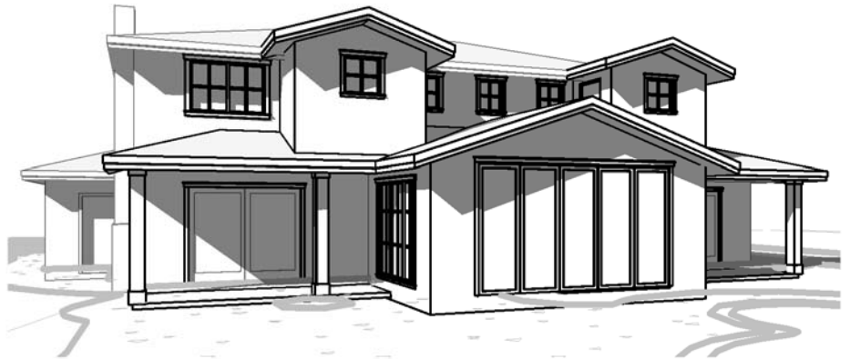
COMPOSITE SHINGLE "CLASS A" ROOF COVERING (LIGHT GREY TO MATCH EXISTING) MANUF.: CERTAINTEED OR SIMILAR
