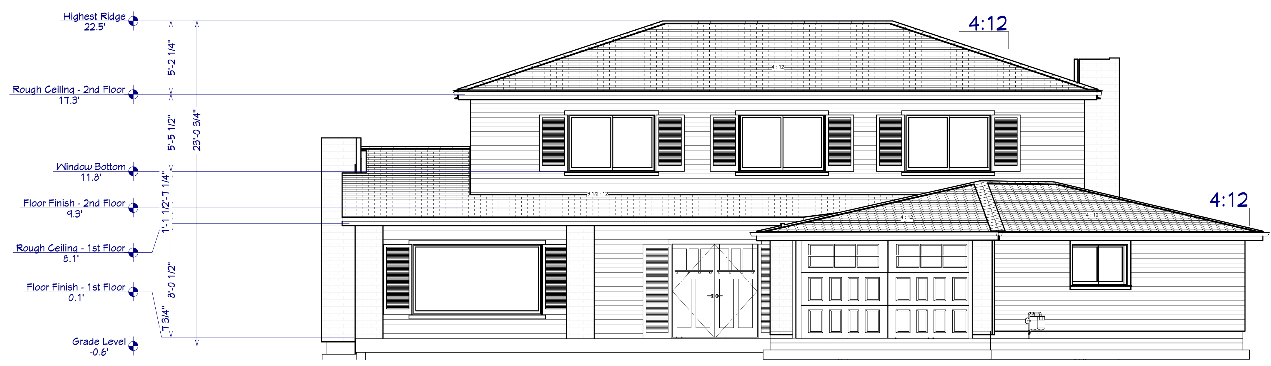
Existing Elevation Front
