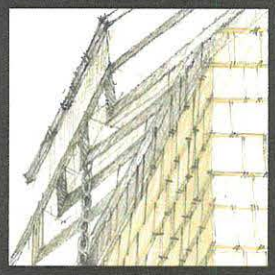
wood trim and rafters Wood trim and exposed rafters, painted white (and window trim)
