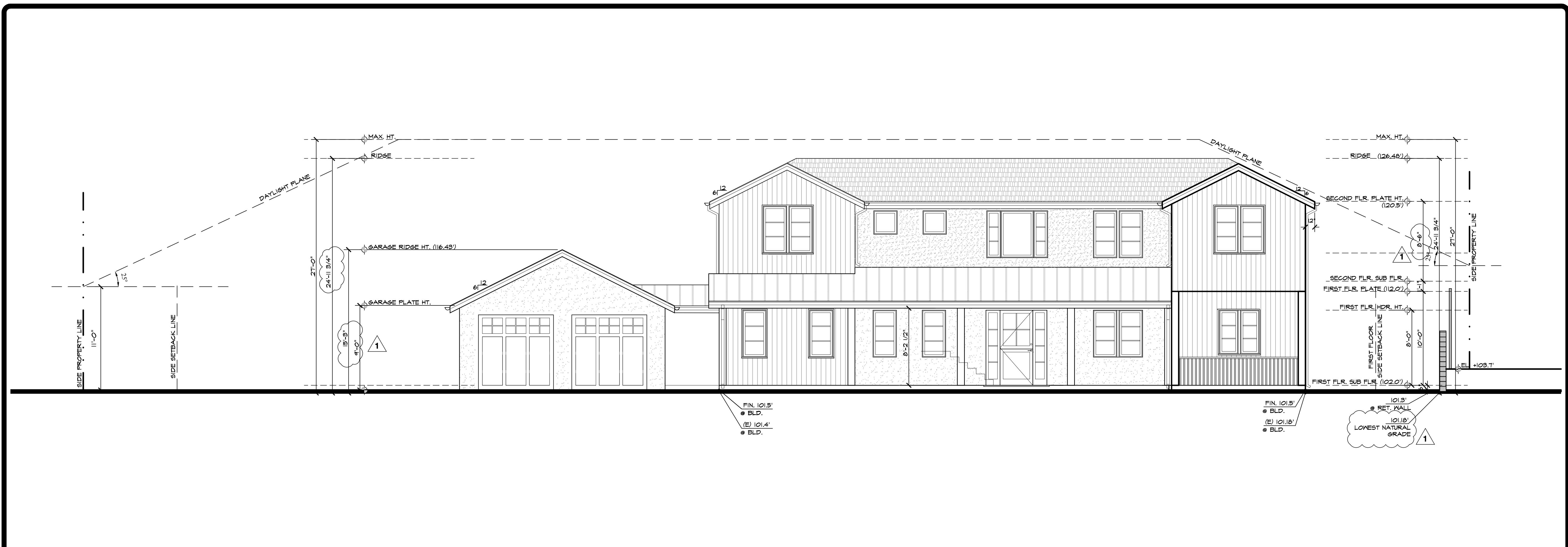
PROPOSED FRONT ELEVATION WITH DAYLIGHT PLANE (reduced scale to fit property lines)
