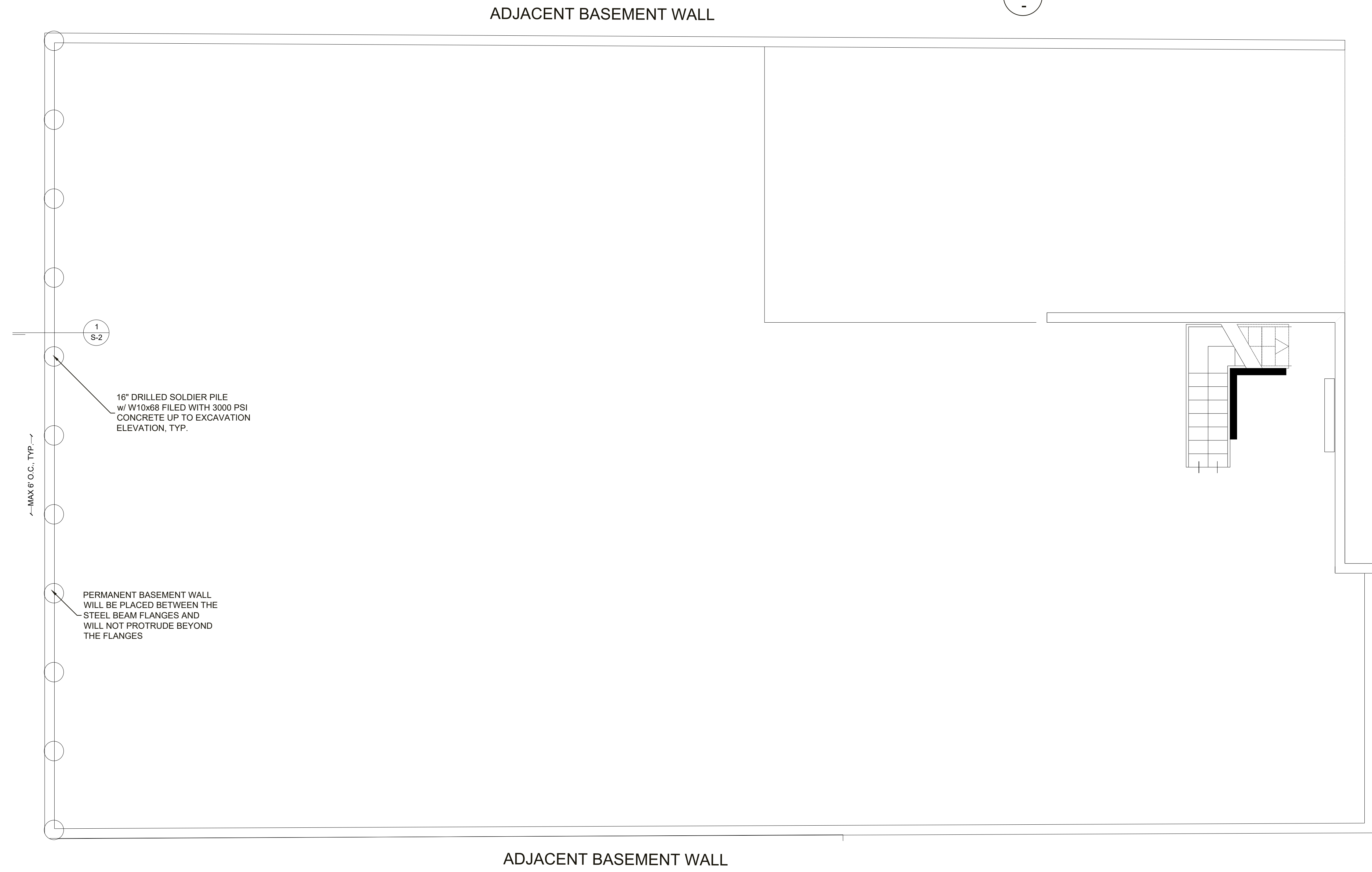
2 SHORING STITCH PILE PLAN VIEW
