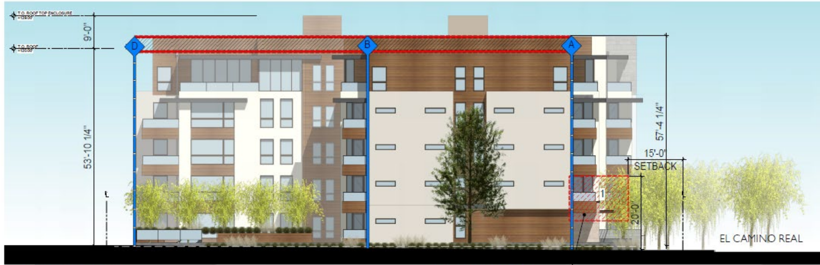
STORY POLE EAST ELEVATION
