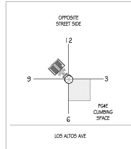
NOTE: FIBER CONNECTION TO BE INSTALLED UNDER SEPARATE PERMIT (N) 7' POLE EXTENSION
