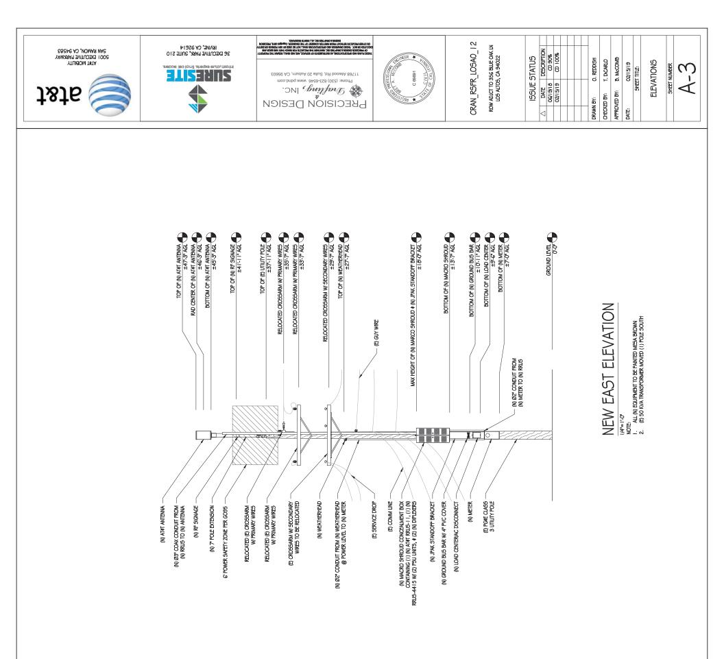
TOP OF (E) INSULATOR ±38-9 AGL TOP OF (E) UTILITY POLE ±37-1 AGL (E) CROSSARM W/ FRIMARY WRES ±37-5 AGL 10P OF (E) TRANSFORMER ±33-9 AGL BOTTOM OF (E) TRANSFORMER ±33-9 AGL E) CROSSARM W/ SECONDARY & SERVICE PROP ±33-9 AGL (E) GUY WRE ±26-9 AGL (E) COMM UNE ±23-10 AGL (E) COMM UNE ±20-9 AGL
