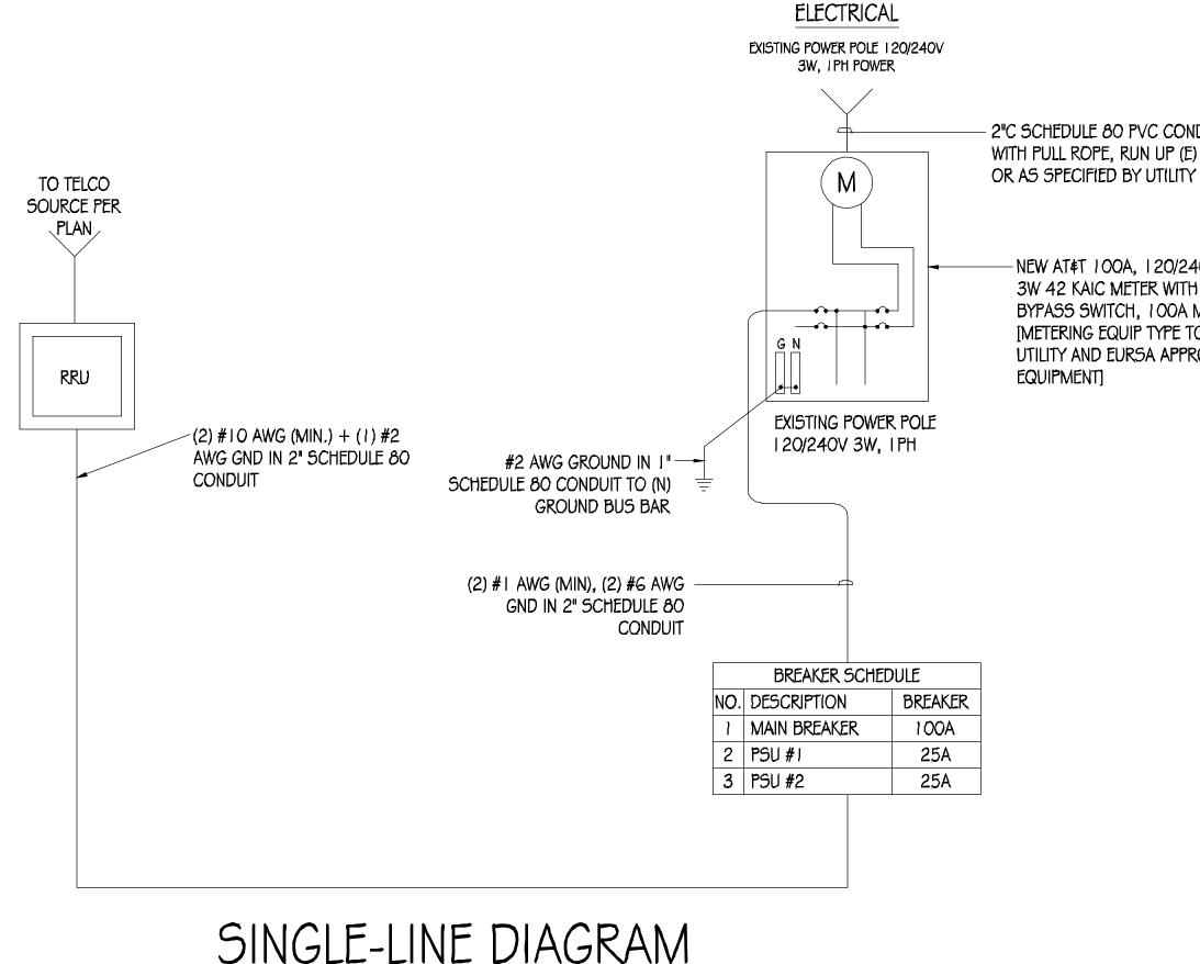
2"C SCHEDULE 80 PVC CONDUIT WITH PULL ROPE, RUN UP (E) POLE
