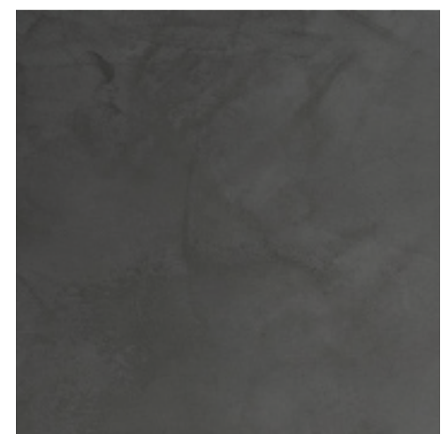
EXTERIOR PLASTER #2 (SMOOTH TROWELED)
