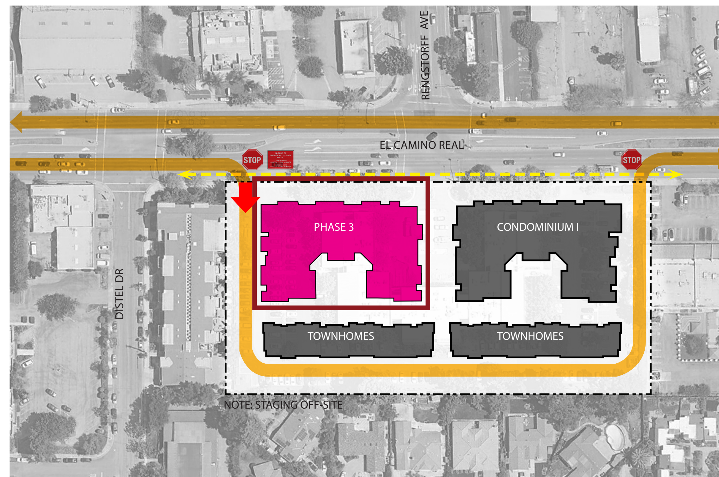
PHASE 3 CONDOMINIUM BUILDING II (UNDERGROUND GARAGE & 5-STORY RESIDENTIAL)
