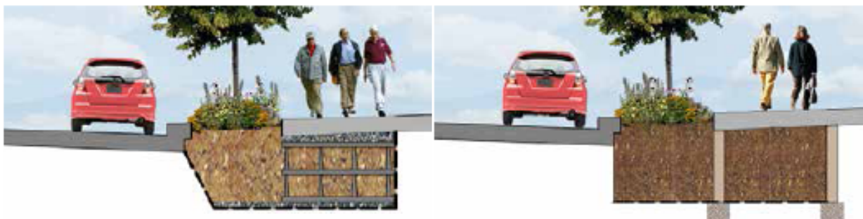
Figure 2-3 Stormwater tree well filter conceptual examples: modular suspended pavement system (left), column suspended pavement system (right) (Courtesy of City of Philadelphia Water Department)
