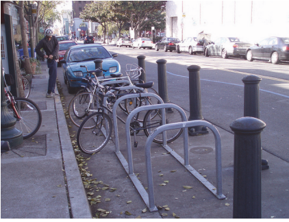
Converted bicycle parking increases parking capacity from one car space to eight bicycle spaces.
